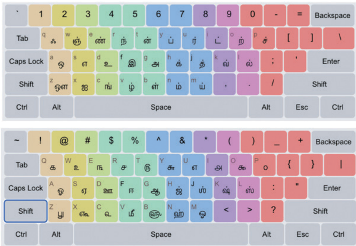
Fig-4. Our proposed Keyboard Layout for regular (top) and shift (bottom) faces
